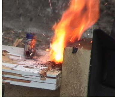
Battery safety testing bullet penetration of AA-size LiFeS 2 cells
